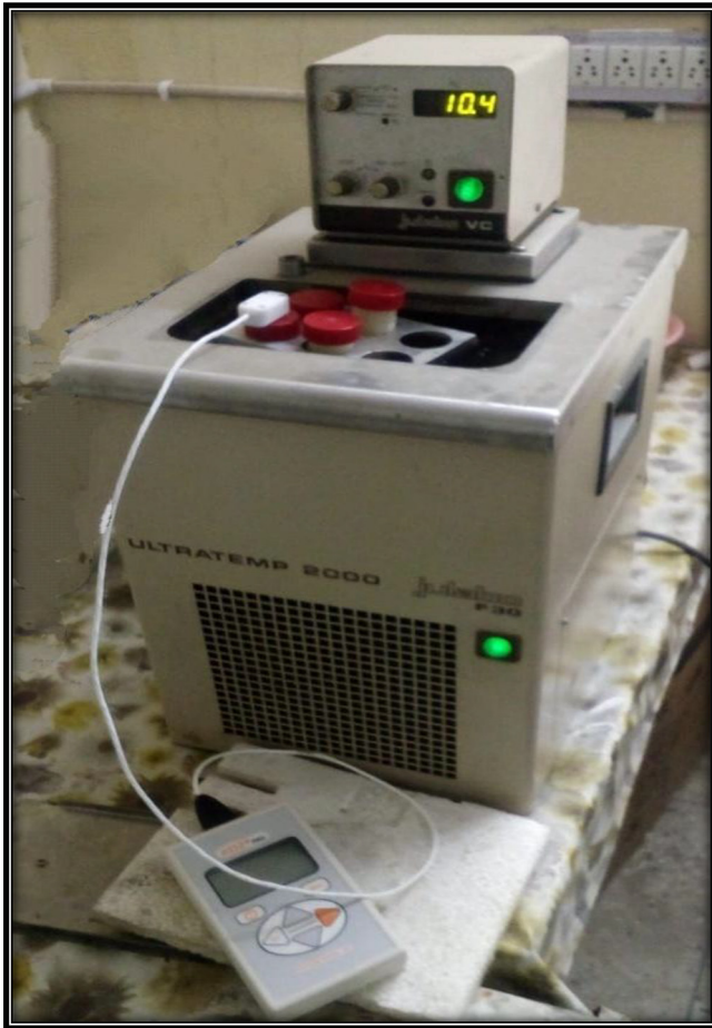
Fig. 6. Circulator setup and thermal conductivity measuring probe.
